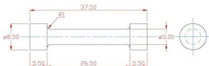
Figure 7 – Tensile test specimen dimensions (dimensions in mm)
