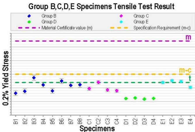
Figure 9 – Tensile test results for Group B, C, D, and E<sup>1</sup>
