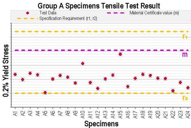
Figure 8 – Tensile test results for Group A specimens<sup>1</sup>
