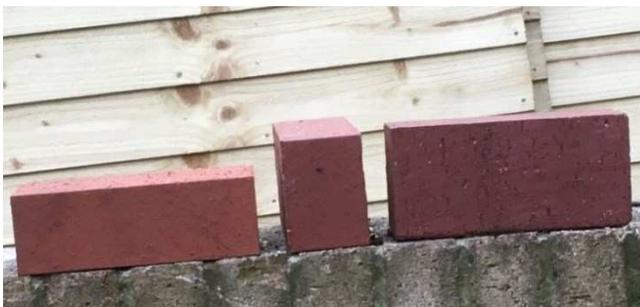
Fig. 5: Bricks used for construction of specimens.
