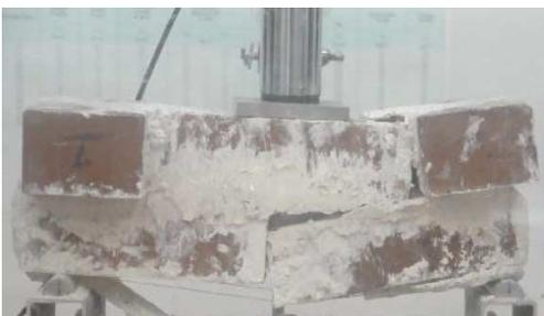
Fig. 17: Failure mode of an unreinforced specimen
