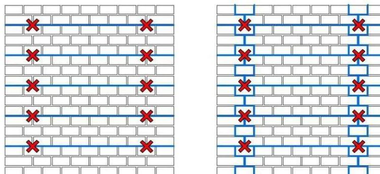
Fig. 21: The reinforcing technique for a masonry wall panel (blue lines: steel cords, red crosses: through connectors).
