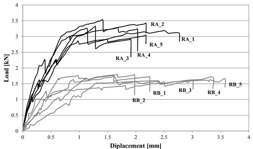
Fig. 18: Load – displacement curves for reinforced samples.
