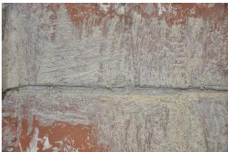
Fig. 10: Excavation manually realized in the horizontal mortar joint.
