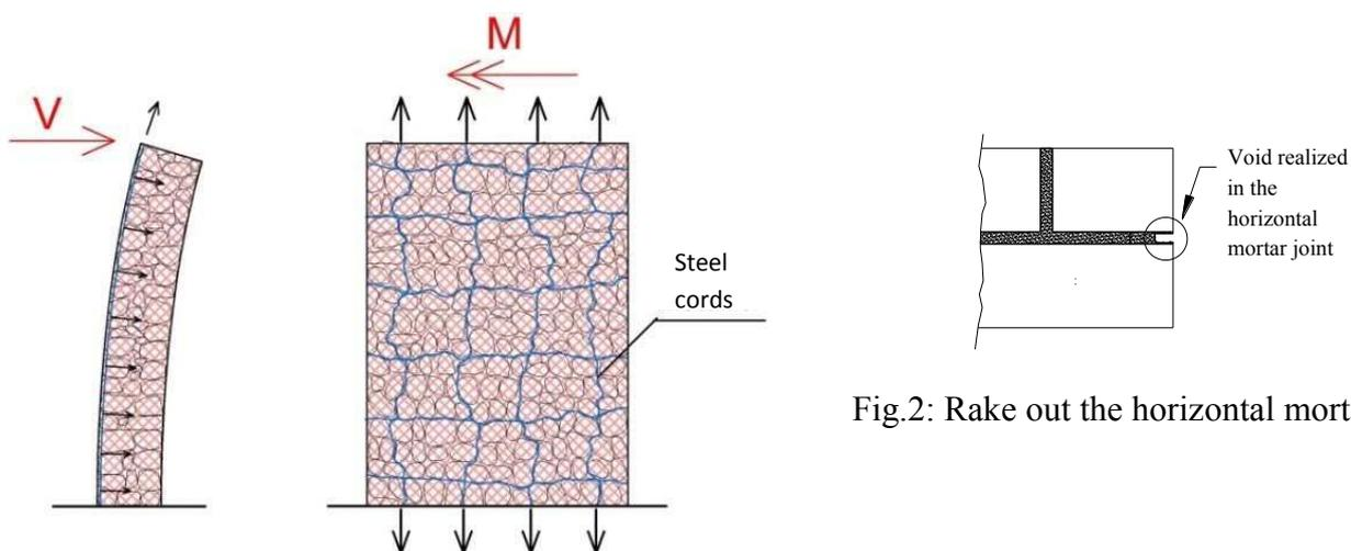
Fig. 1: Mechanical behavior of the reinforcement.
