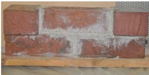
Fig. 8: Unreinforced specimens.
