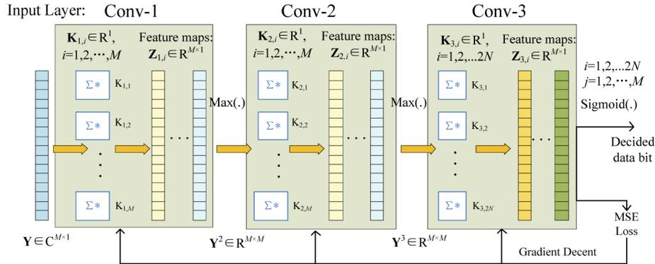
Fig. 2. The structure of CNN based demodulator.
