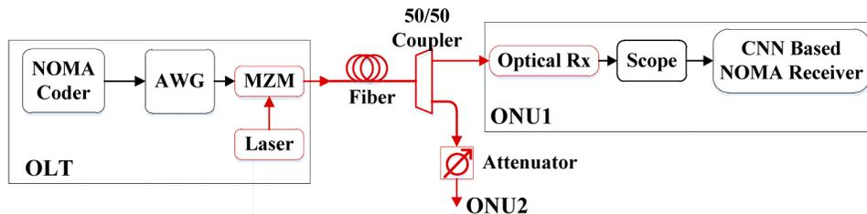
Fig. 3. Experiment setup for NOMA-PON with two ONUs.
