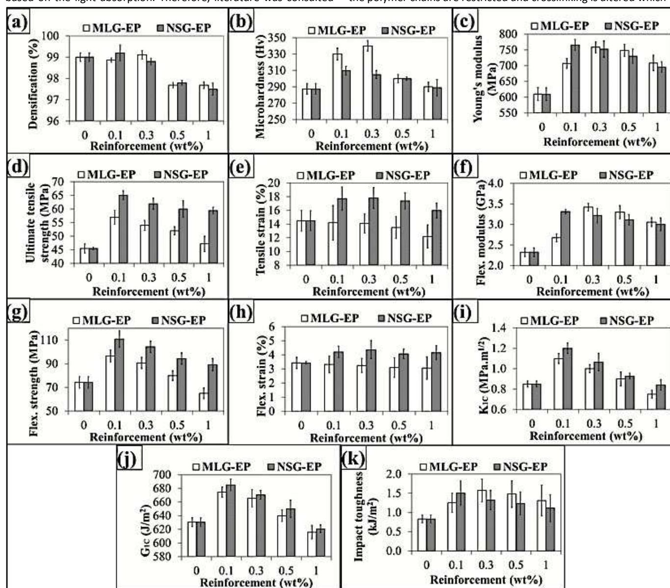
Fig. 4 Densification and mechanical properties: (a) densification, (b) microhardness (Hv), (c) Young's modulus, (d) ultimate tensile strength, (e) tensile strain (%), (f) flexural modulus, (g) flexural strength, (h) flexural strain (%), (i)  $K_{IC}$ , (j)  $G_{IC}$  and (k) Charpy impact toughness.
