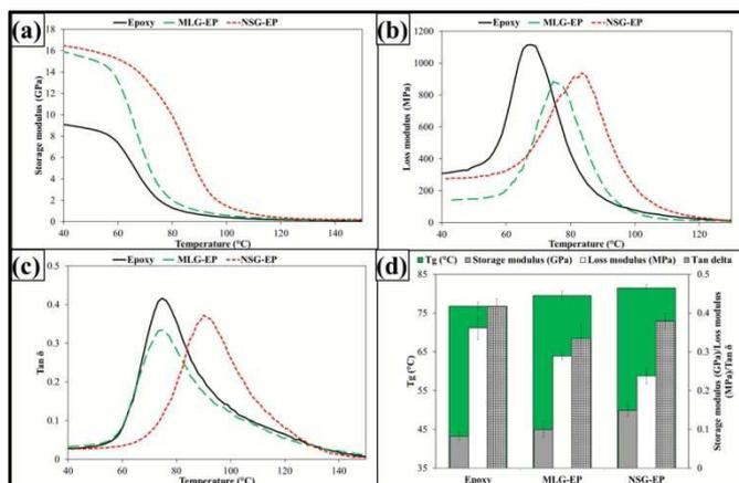
Fig. 5 Dynamic mechanical properties: (a) storage modulus, (b) loss modulus, (c)  $\text{Tan}\delta$ , and (d)  $T_g$ , and values of storage modulus, loss modulus and  $\text{Tan}\delta$  at  $T_g$ .
