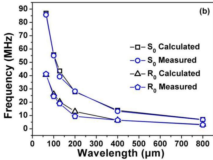
Fig. 2 Comparison of calculated and measured frequencies of  $A_0$  modes (a);  $R_0$  and  $S_0$  modes (b) for the devices with different wavelengths.
