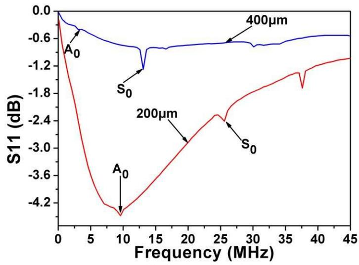
Fig. 1 Frequency response (S11) spectra of the Al foil SAW devices with different wavelengths (200 and 400 μm).
