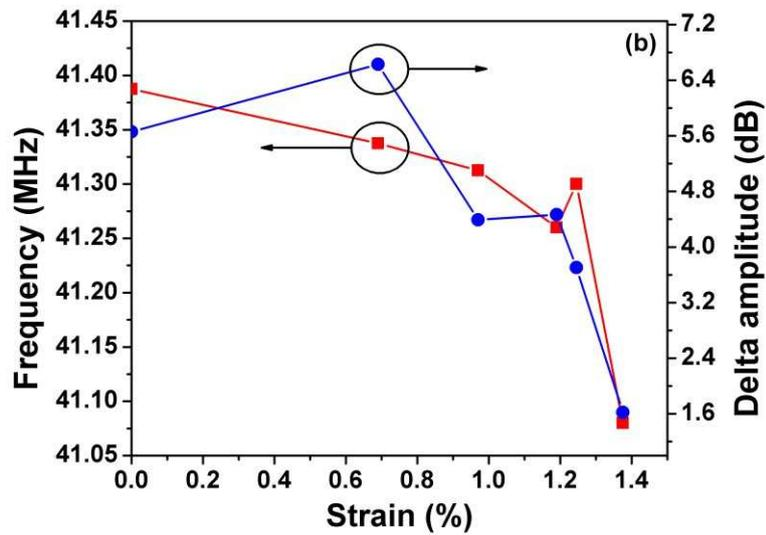
Fig. 3 (a) Comparison of transmission signals  $S_{12}$  of a device with bending strain of 0%, 1.375% and its return to flat shape; the embedded photo shows a side view of a bent Al foil SAW device at a maximum strain 1.375% when  $\theta \cong 90^\circ$ ; (b) The relationships among bending strain, amplitude peak height and frequency shift.
