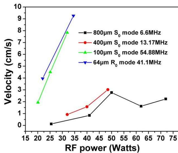
Fig. 6 Velocities of the droplet (2.5 uL) movement versus input power for devices with different wavelengths.
