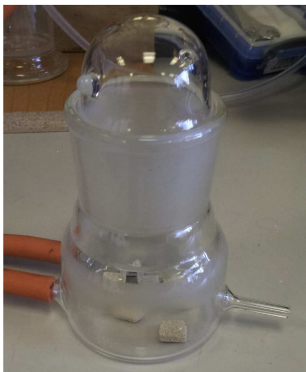
Fig. 1. Image of the glass reactor. Reactor diameter 78 mm for scale.
