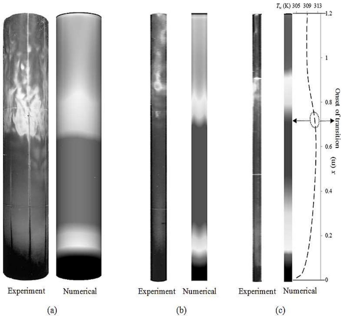
Fig. 4. Temperature distribution along the cylinder surface. (a)  $D = 165$  mm, (b)  $D = 26$  mm, and (c)  $D = 10$  mm.
