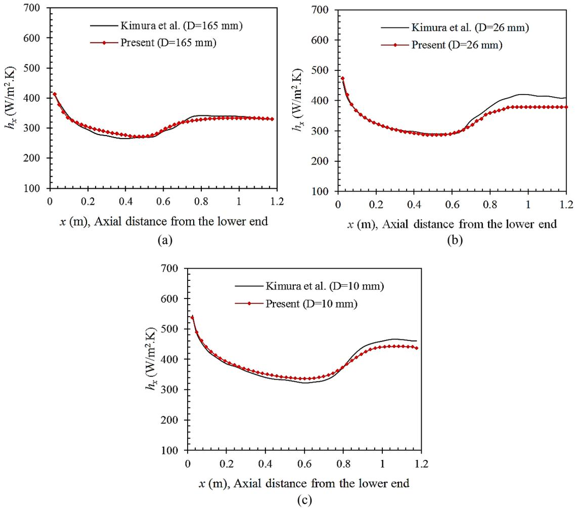
Fig. 5. Comparisons of local heat transfer coefficient between the present work and data for Kimura et al. [xx] for different diameters (a)  $D=165$  mm, (b)  $D=26$  mm, and (c)  $D=10$  mm.
