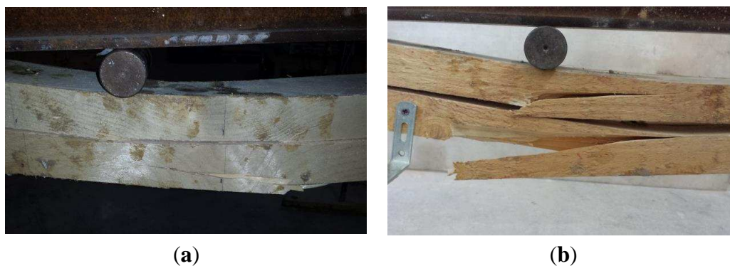
Figure 10. Timber tensile-flexural failures (beams that were cut in half): (a) in the lower half; (b) both in the lower and upper half.
