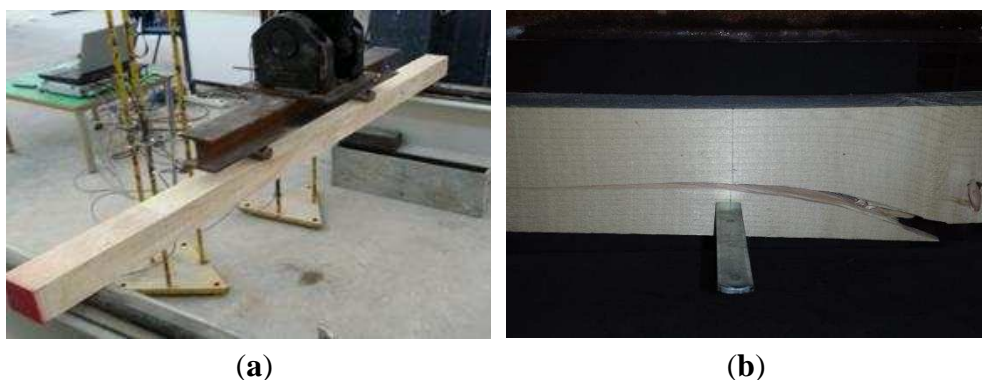
Figure 5. (a) Four-point-bending test setup; (b) Typical tensile failure mode of control beams near a knot or due to grain deviation.
