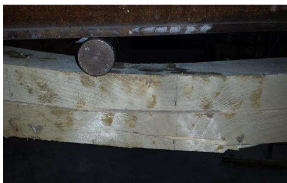
Figure 10. Timber tensile-flexural failures (cut in half beams): (a) in the lower half; (b) both in the lower and upper half.
