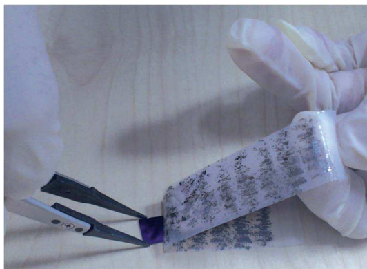
Fig. 2 Scotch tape method of graphene synthesis from graphite block. 39 Reproduced with permission from ref. 39.
