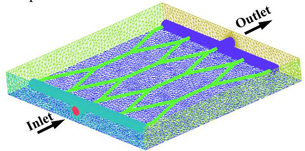
Figure 11: Computational domain. Figure 12 shows the profiles of contour temperature, pressure and velocity of a new MCHS at steady state when a constant water inlet temperature (293 K), mass flow rate (1.0 L/min) and heat flux ( $5.0 \times 10^5 \text{ W/m}^2$ ) is applied.
