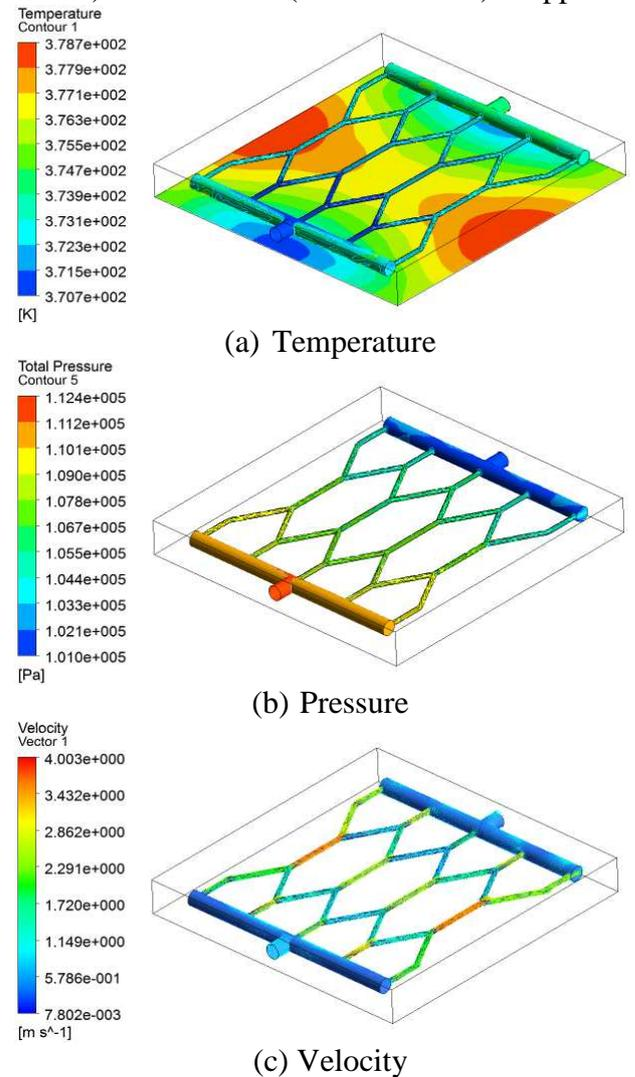
Figure 12: (a) Temperature, (b) pressure and (c) velocity profile of a new MCHS. It is found from Figure 12 (a) that more stable distribution of temperature is achieved for the new design of MCHS. This heat sink design can
