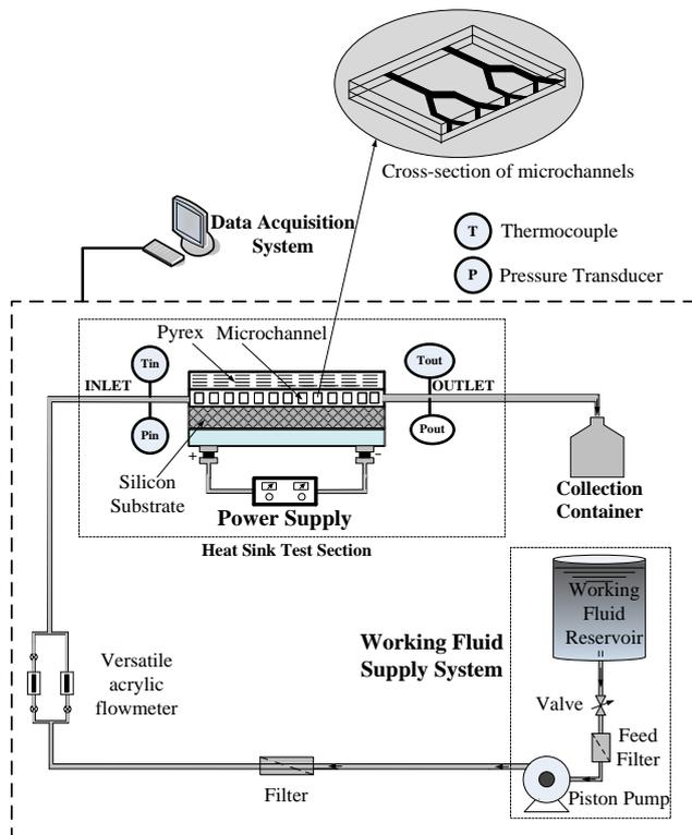
Figure 1. The schematic diagram of the experimental apparatus.
