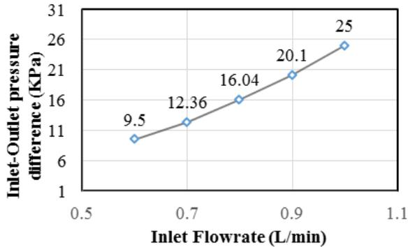
Figure 6: Pressure drop vs flow rate.
