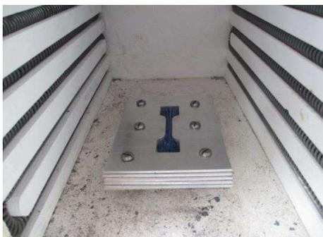
Fig. 1. Specimen mould in oven
