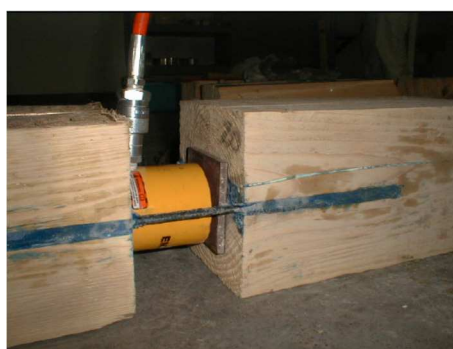
Figure 7. Pull-out test arrangement (tests without strain gauges).
