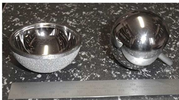
Figure 1 DePuy ASR™ resurfacing hip (note the small femoral stem right). To the left is the acetabular cup and to the right is the single-piece femoral component.
