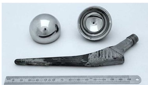
Figure 2 DePuy ASR™ XL total hip replacement with conventional femoral stem (shown above ruler). Femoral head is shown top left and the acetabular cup is shown top right.
