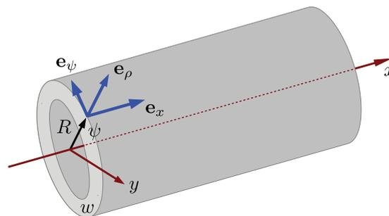
Fig. 1: (Colour on-line) A sketch of a nanotube with an outer radius  $R$  and an inner radius  $R - w$ . A point on the outer surface of the nanotube is parametrized by the coordinate  $x$  along its symmetry axis and the polar angle  $\psi$ . The unit vectors  $\mathbf{e}_x$  (parallel to the symmetry axis),  $\mathbf{e}_\psi$  (tangential to the surface), and  $\mathbf{e}_\rho$  (normal to the surface) form a right-handed triplet.
