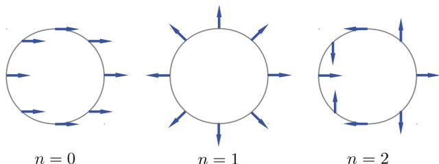
Fig. 4: (Colour on-line) Magnetization in a cross-section of the nanotube for different helicities  $n$ . The case  $n = 0$  corresponds to a transverse domain wall [26].
