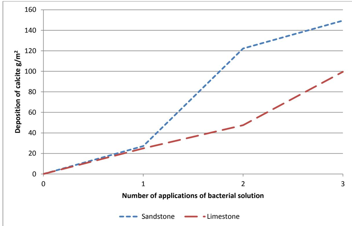
Figure 3 – Comparison of calcite deposition
