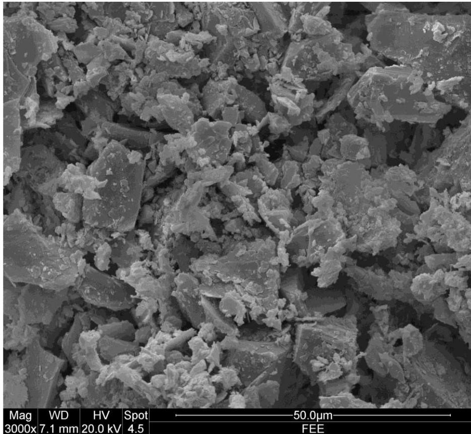
Figure 5 – Sandstone displaying calcite deposition after three surface applications (3000 x magnification).
