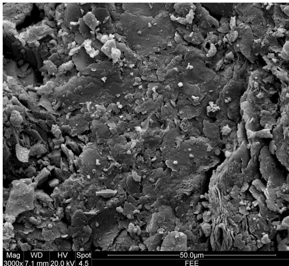
Figure 4 – Untreated sandstone control sample (3000 x magnification)
