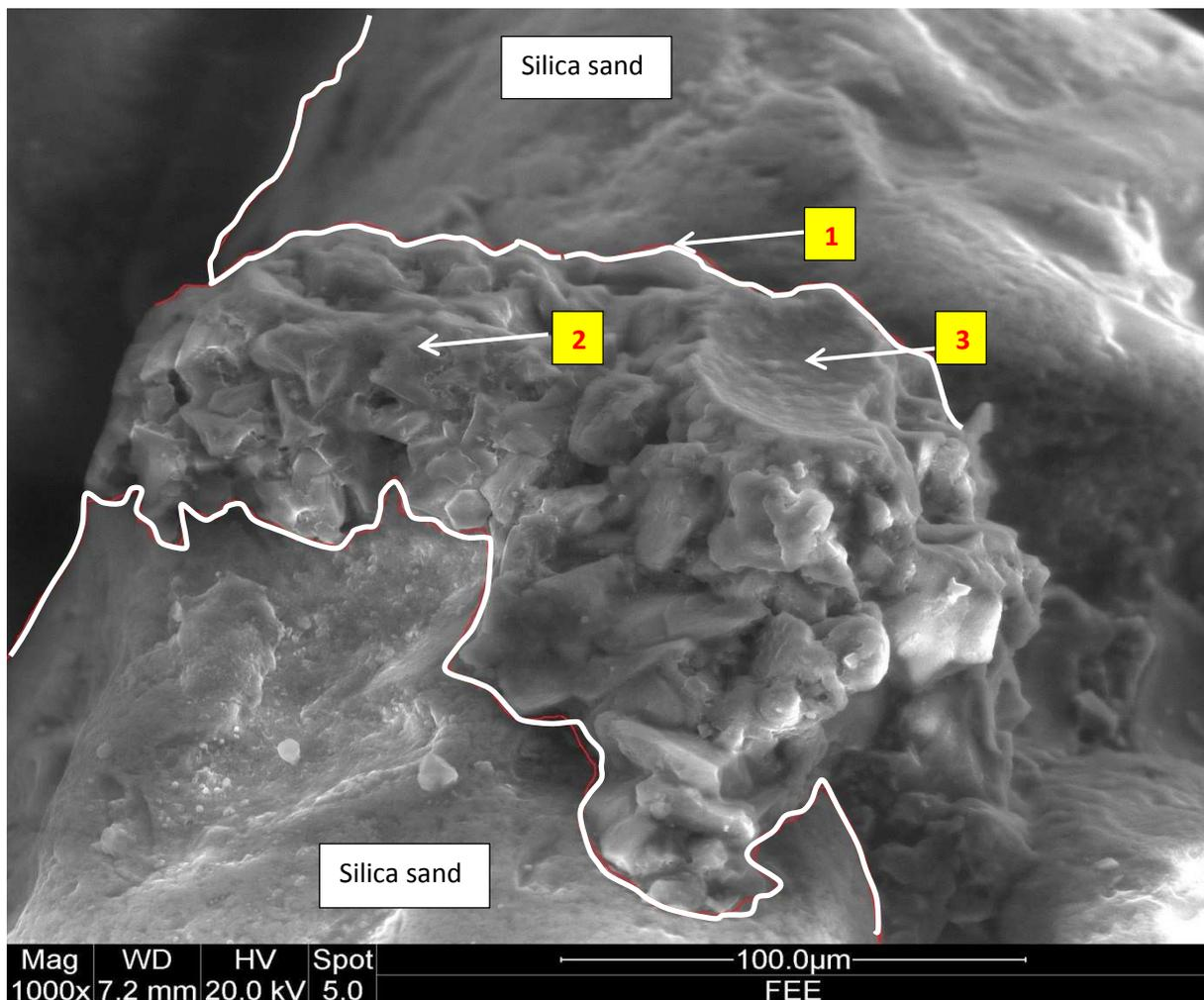
Figure 6 Calcite formation bonding sand grains 1000 x magnification).
