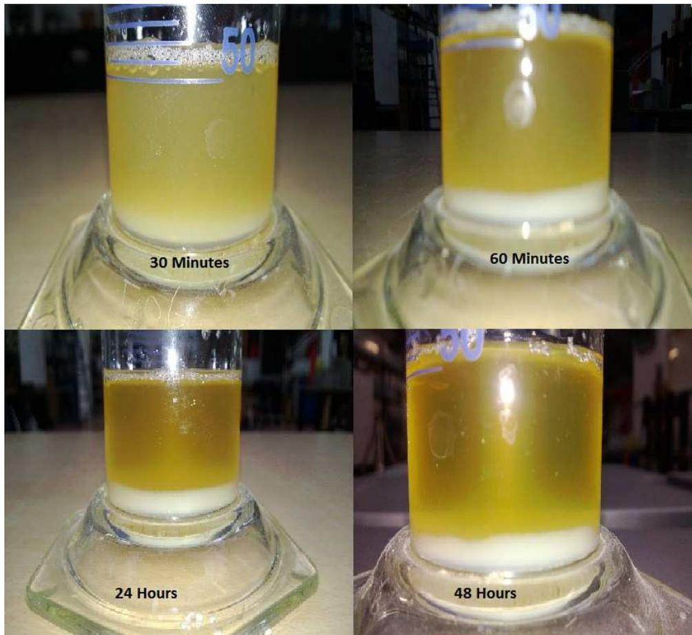
Figure 2 - The sequence of calcite precipitation from the two reactants.
