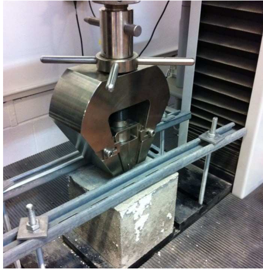
Figure 3. - Pull out testing arrangement of Lloyds testing apparatus
