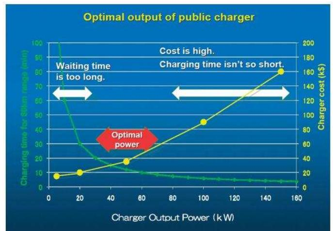
Figure 1. Optimal output of fast charger [5]
