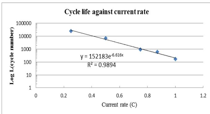
Figure 2. battery cycle life at different current rates
