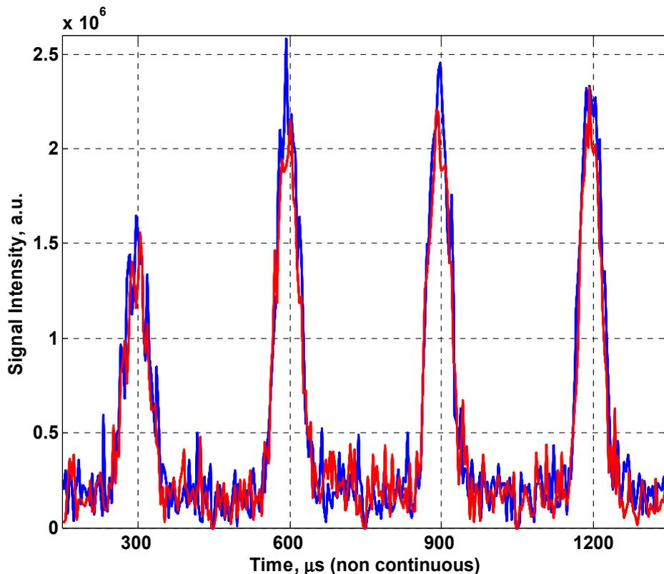
**Figure 8.** Normalized data for a saturation recovery sequence for the red palm oil used a 128 echo train and 512 averages. Data for the flat fabric coil is shown as red circles whilst the fabric coil wrapped round the 8 cm tube is shown as blue squares.
