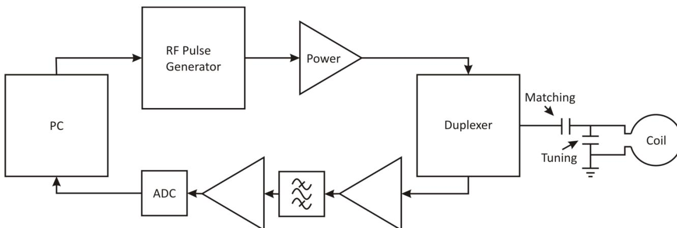
The NMR probe usually consists of a coil with a tuning capacitor in parallel with the coil and, a matching capacitor in series with the coil, allowing the probe to apply and receive high frequency
