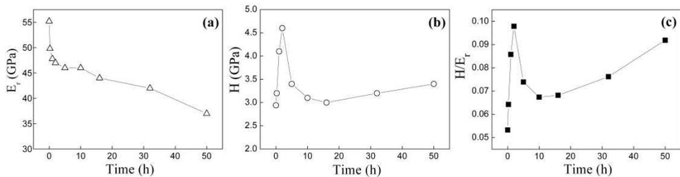
**Figure 5.** Dependence of (a) reduced Young's modulus,  $E_r$ , (b) hardness, H and (c)  $H/E_r$  ratio on the immersion time in HBBS at 37°C for  $Mg_{72}Zn_{23}Ca_5$  alloy. Adapted and reprinted from Pellicer et al. [77], page 8, with permission from John Wiley&Sons.
