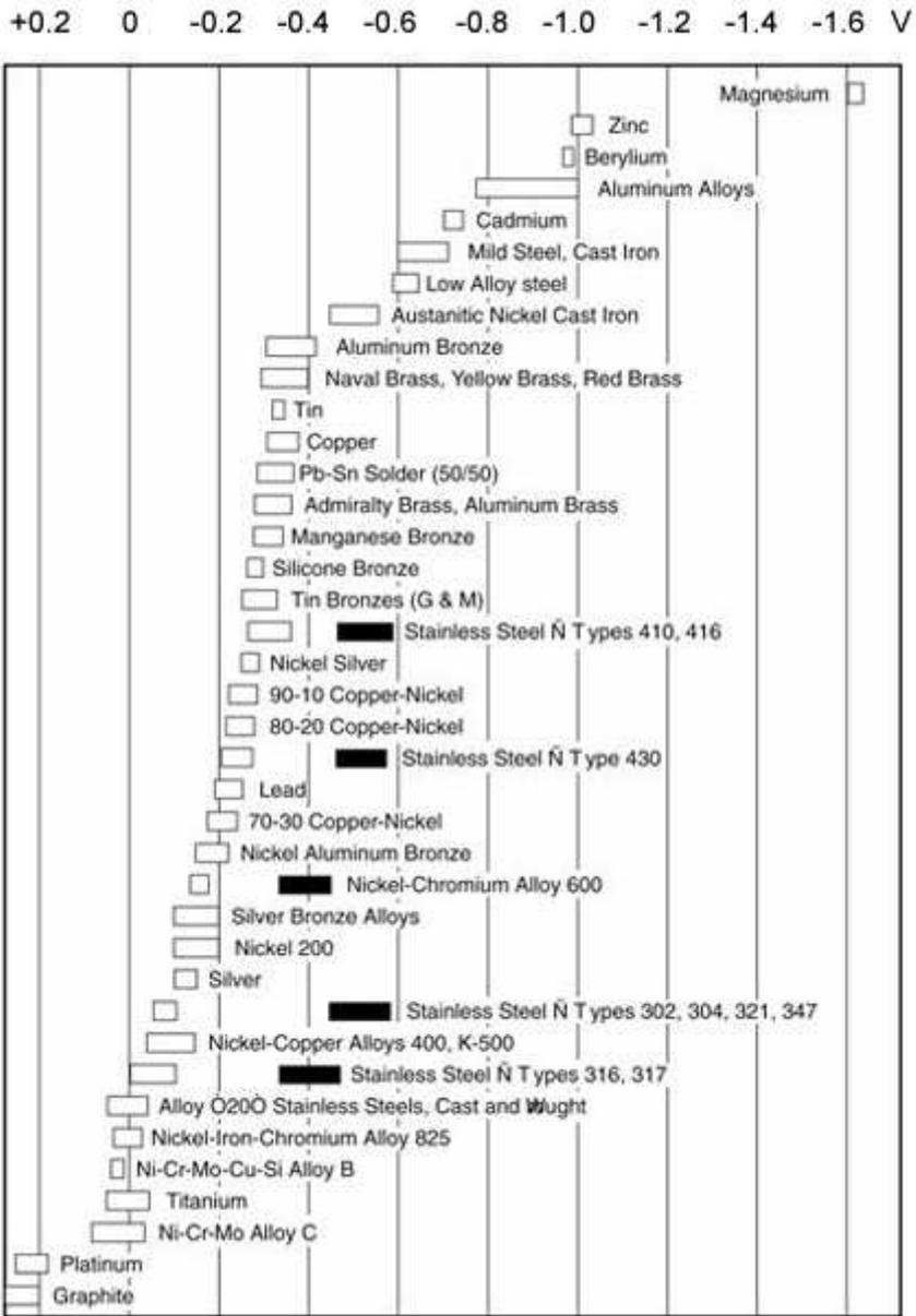
**Figure 3.** The galvanic series of metals, semi-metals and alloys of industrial interest showing their potentials (in volts) in flowing sea water, arranged from the most noble (bottom) to the most active (top) material. The values are referred to saturated calomel half-cell reference electrode. Adapted and reprinted from Amtec Consultants [27]
