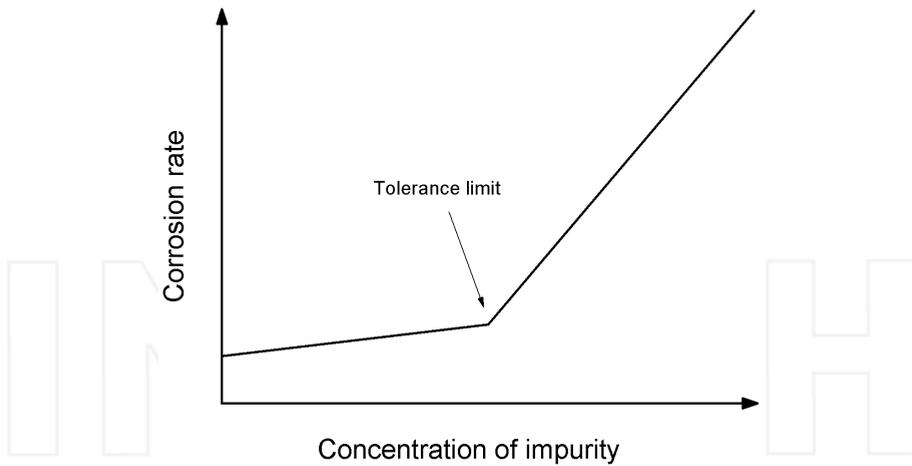
**Figure 4.** Schematic picture showing the dependence of the impurity concentration on the corrosion rate of Mg. The tolerance limit sets the threshold between the region for which an increase of the impurity concentration hardly affects the corrosion rate (left) and the region for which a further increase of the impurity concentration abruptly increases the corrosion rate.
