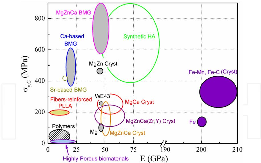
**Figure 6.** Comparison of the mechanical properties (compressive yield stress,  $\sigma_{y,C}$  versus Young's modulus, E) in linear scale for different families of biodegradable implant materials, including metallic alloys (Mg-based, Ca-based, Sr-based, or Fe-based), ceramics (e.g., synthetic hydroxyapatites) and polymers. Adapted and reprinted from Pellicer et al. [77], page 13, with permission from John Wiley&Sons.
