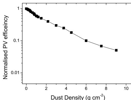
Figure 7: Experimental data from an investigation of the effect of sand and dust accumulation on PV module performance in Kuwait by Al-Hasan [1].
