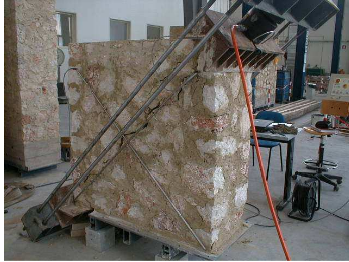
Fig. 1 Typical layout of a diagonal compression test.
