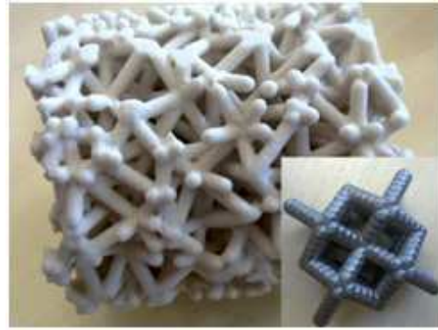
Figure 3: Randomised and regular (in inset) geometry structures
