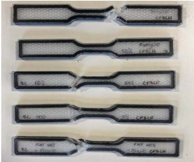
Fig. 4. Fatigue testing and failed samples
