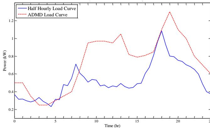
Fig. 4 Comparison of half hourly winter load curve
