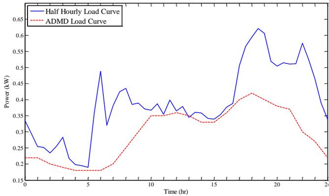
Fig. 3 Comparison of half hourly summer load curve
