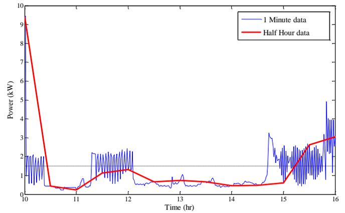
Fig. 2 Comparison of 1Minute and 30 Minute time resolution with 1.5 kW on-site generation
