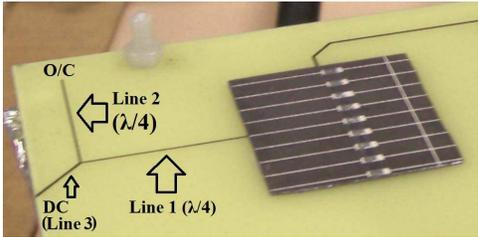
Figure 2. The DC/AC decoupling circuit.
