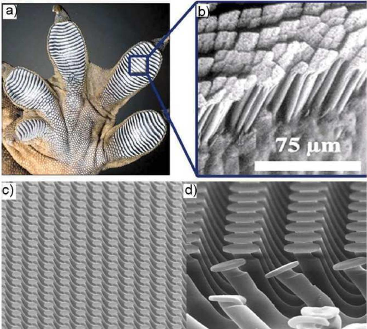
**Figure 3** Gecko Feet Showing Structure and polymeric analogues a) Gecko foot b) setae (From L. Ge et al., PNAS **104**, 10792-10795, 2007). c) and d) polymeric analogues (From D. Sameoto and C. Menon, J. Micromech. Microeng. **20**, 115037, 2010, IOP publishing, reproduced by permission).
