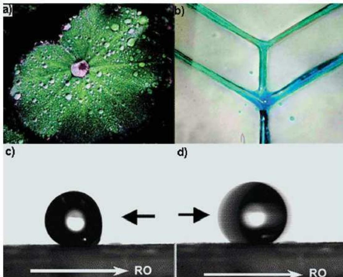
**Figure 6** a) *Alchimilla mollis* leaf b) patterned superhydrophobic surface (From N.J. Shirtcliffe et al., *Langmuir* **25**, 14121-14128, 2009, ©American Chemical Society, reproduced by permission) and c) and d) directional anisotropy of butterfly wings, the drop moves to the right but not to the left even though the driving force is the same (From Y. Zheng et al., *Soft Matter* **3**, 178-182, 2007, The Royal Society of Chemistry, reproduced by permission).
