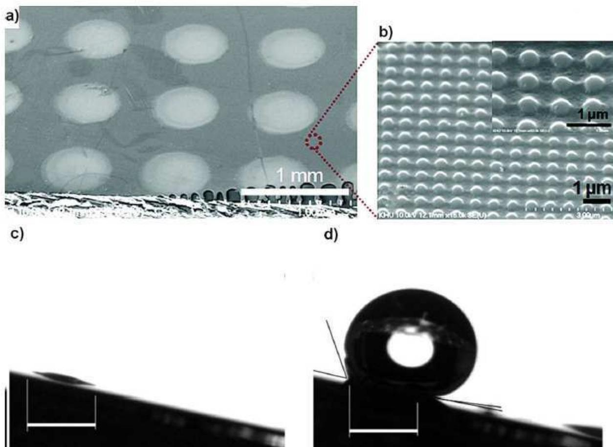
**Figure 7** Polymeric fog capture surfaces a) low magnification image showing hydrophilic spots b) high magnification image showing superhydrophobic structure (From J. Choi et al., *Langmuir* **25**, 7156-7160, 2009, ©American Chemical Society<sup>129</sup>), c) and d) dewetting of drops from a patterned superhydrophobic surface (From C. Dorrer and J. Ruhe, *Langmuir* **24**, 6154-6158, 2008, ©American Chemical Society).
