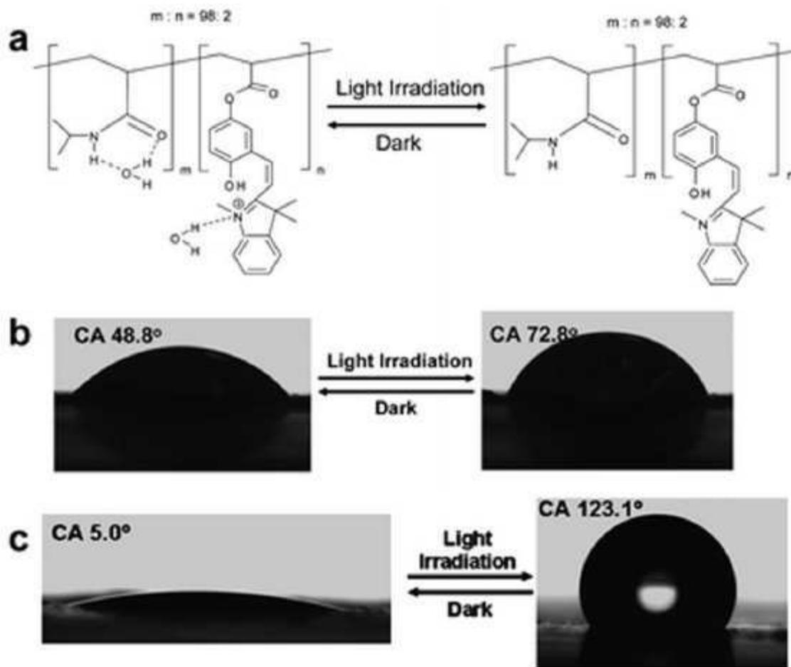
**Figure 8** a) Chemical switch activated by light b) flat contact angle change c) rough contact angle change (From G. Joseph et al., *Analyst* **135**, 2303-2308, 2010, The Royal Society of Chemistry, reproduced by permission).
