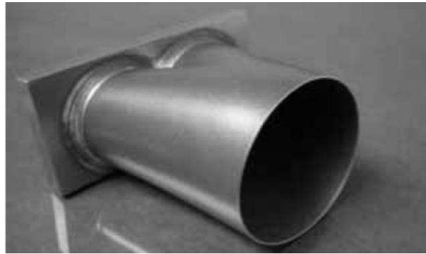
Fig. 8 Motorsport exhaust fabricated via Accufusion laser consolidation process 10
