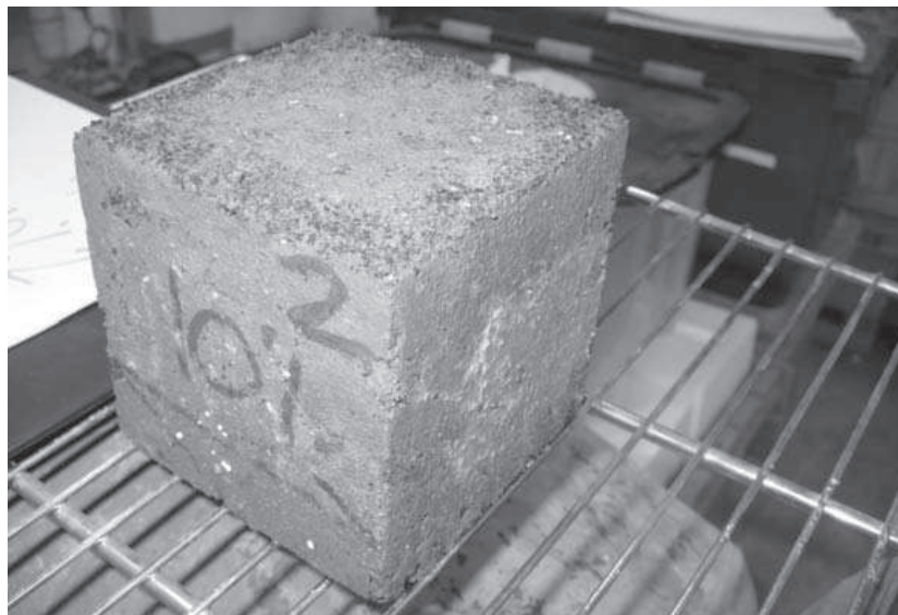
Plate 4: 10% Rubber sample at 50 freeze/thaw cycles
