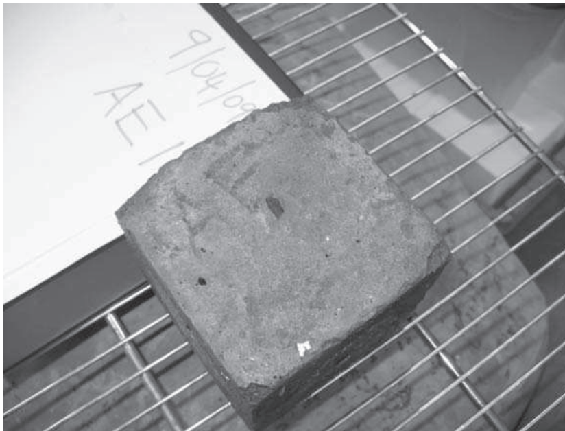
Plate 2: Air Entrained sample at 50 freeze/thaw cycles
