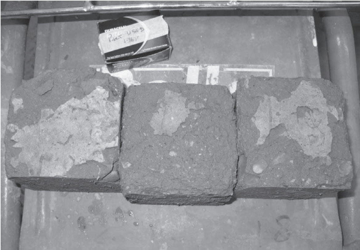
Plate 1: Plain concrete cubes at 50 freeze/thaw cycles
