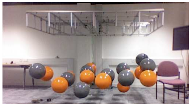
Figure 4: The chassis frame that was built to support the matrix of spheres
