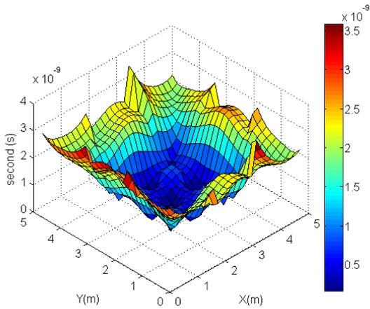
Fig.7. Distribution of RMS delay spread for four transmitters. The positions of the transmitters are (1.25, 1.25), (1.25, 3.75), (3.75, 1.25), (3.75, 3.75) with the LED semiangle of 30 degree.
