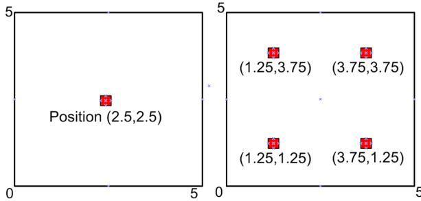
Fig. 2. The position of transmitters on the ceiling.
