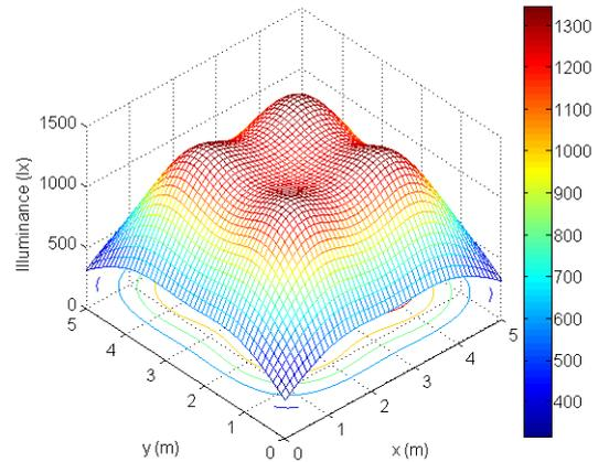
Fig. 5. Distribution of illuminance with 4 transmitters with the LED semiangle of 70 degree. Max= 1342.50 lx; Min=315.90 lx; Average=958.11 lx.
