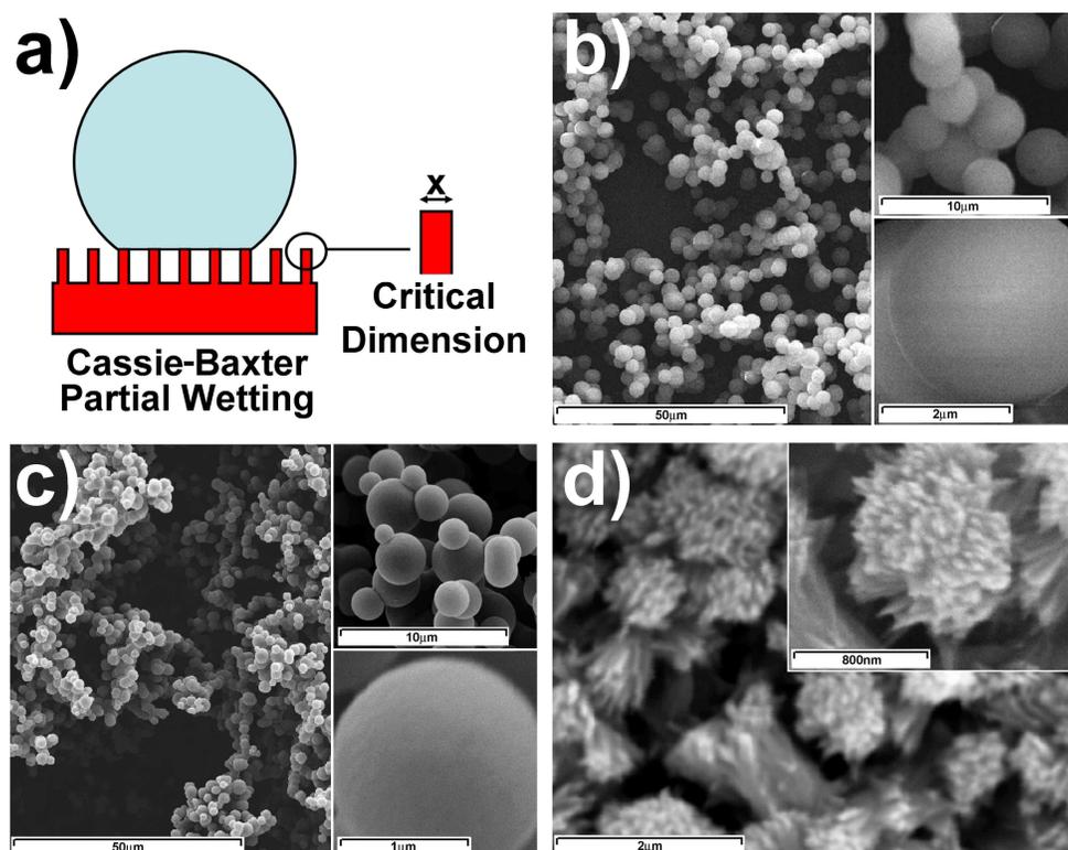
**Fig. 1** (a) Diagram showing Cassie-Baxter superhydrophobicity and the critical dimension used to define surfaces here. Electron micrographs of (b) the larger scale sol-gel material, (c) the smaller scale sol-gel and (d) the copper oxide nano-pillars.
