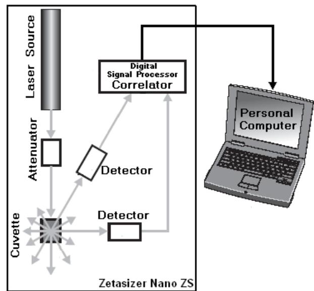
Figure 3. Schematics of Zetasizer nano-particle analyzer [34]
