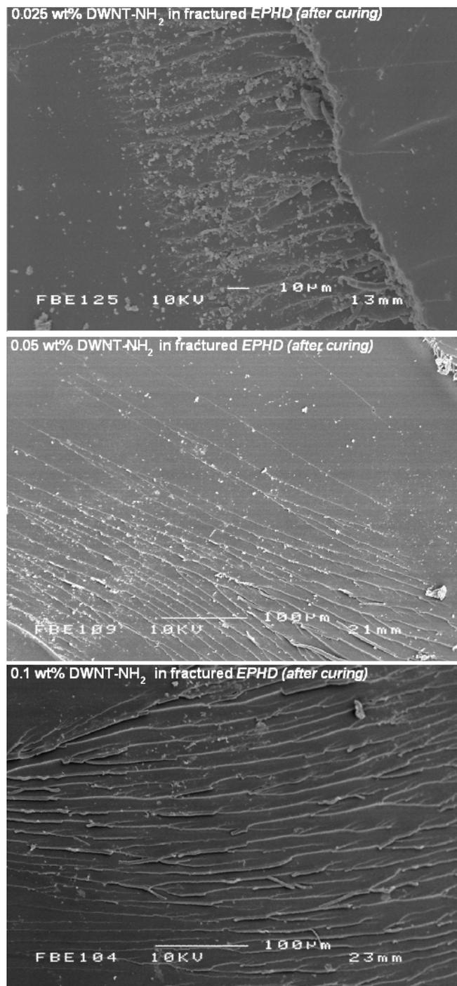
Figure 5. Representative fractured surfaces of cured nanocomposite
