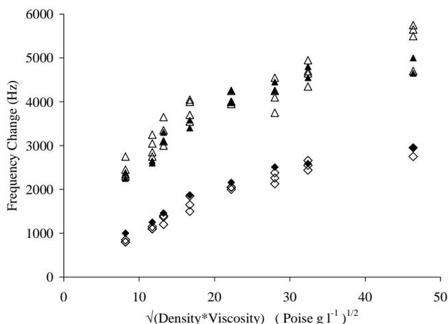
**Fig. 3.** Change in resonant frequency as a function of the square root of the density-viscosity product for 3  $\mu\text{m}$  thick flat surfaces without hydrophobic treatment (open diamonds), 3  $\mu\text{m}$  thick flat surfaces with hydrophobic treatment (solid diamonds), 3  $\mu\text{m}$  tall patterns without hydrophobic treatment (open triangles) and 3  $\mu\text{m}$  tall patterns with hydrophobic treatment (solid triangles).
