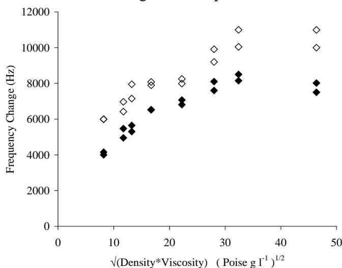
**Fig. 4.** Change in resonant frequency as a function of the square root of the density-viscosity product for 5  $\mu\text{m}$  tall patterns without hydrophobic treatment (open diamonds) and 5  $\mu\text{m}$  tall patterns with hydrophobic treatment (solid diamonds).
