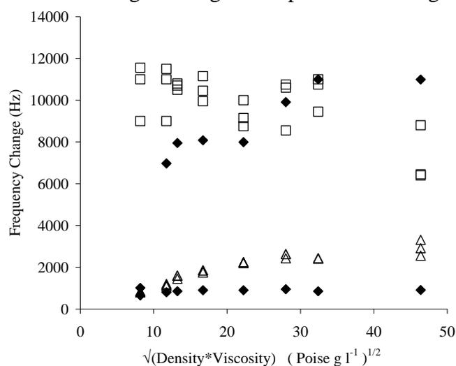
**Fig. 5.** Change in resonant frequency as a function of the square root of the density-viscosity product for 10  $\mu\text{m}$  thick flat surfaces without hydrophobic treatment (open triangles), 10  $\mu\text{m}$  tall patterns without hydrophobic treatment (open squares) and 10  $\mu\text{m}$  tall patterns with hydrophobic treatment (solid diamonds).
