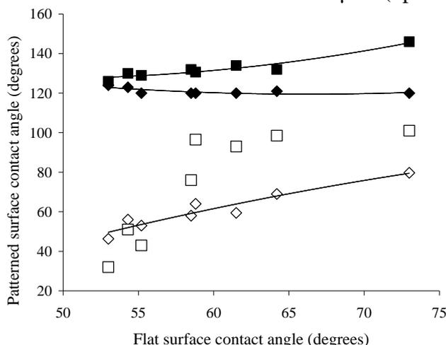
**Fig. 2.** Contact angles for different concentrations of PEG on smooth and patterned surfaces without hydrophobic coating; 3  $\mu\text{m}$  tall (open diamonds) and 10  $\mu\text{m}$  tall (open squares) and with hydrophobic coating 3  $\mu\text{m}$  tall (solid diamonds) and 10  $\mu\text{m}$  tall (solid squares).
