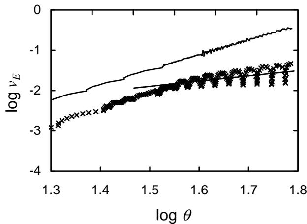
FIG. 2. A log-log plot of the edge speed-dynamic contact angle relationship for a polydimethylsiloxane droplet on a surface with 15  $\mu\text{m}$  diameter pillars of height 45  $\mu\text{m}$  and lattice parameter 30  $\mu\text{m}$  ( $\times\times\times$  symbols); the slope of this data during the initial spreading ( $p=1.296$ ) is also shown. The upper solid curve with a slope of  $p=3$  is data for a smooth surface (shifted upwards by 0.5 for clarity).
