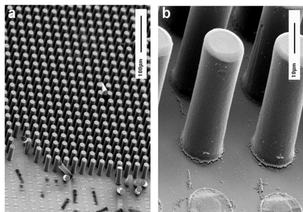
FIG. 1. Scanning electron microscope images of lithographically structured surfaces showing a square lattice of  $15\ \mu\text{m}$  diameter cylindrical pillars with a  $30\ \mu\text{m}$  lattice parameter: (a) view of a field of pillars, and (b) close-up view of the pillars.
