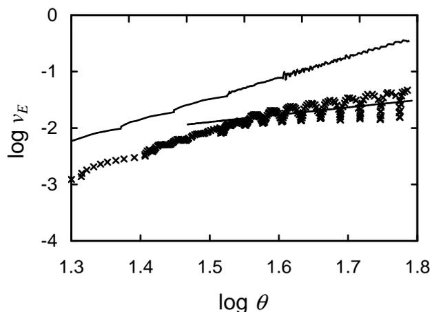
FIG. 2. A log-log plot of the edge speed-dynamic contact angle relationship for a polydimethylsiloxane droplet on a surface with 15  $\mu\text{m}$  diameter pillars of height 45  $\mu\text{m}$  and lattice parameter 30  $\mu\text{m}$  (xxx symbols); the slope of this data during the initial spreading ( $p=1.296$ ) is also shown. The upper solid curve with a slope of  $p=3$  is data for a smooth surface (shifted upwards by 0.5 for clarity).
