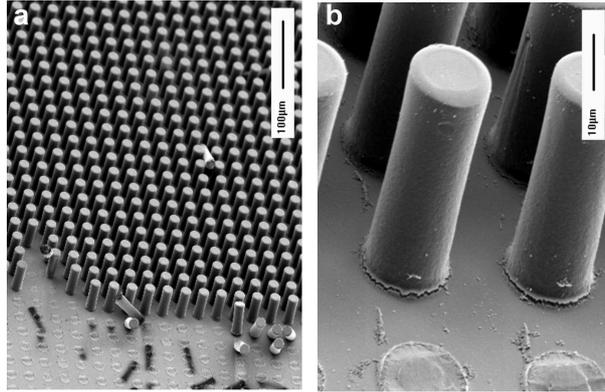
FIG. 1. Scanning electron microscope images of lithographically structured surfaces showing a square lattice of 15  $\mu\text{m}$  diameter cylindrical pillars with a 30  $\mu\text{m}$  lattice parameter: (a) view of a field of pillars, and (b) close-up view of the pillars.
