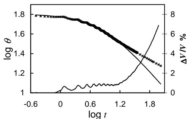
FIG. 3. A log-log plot of the dynamic contact angle and time with a fit of  $\theta \propto 1/(t+t_0)^{0.614}$  for the experiment on the textured surface corresponding to the data in Fig. 2. The percentage change in drop volume is also shown (lower curve and right-hand axis).
