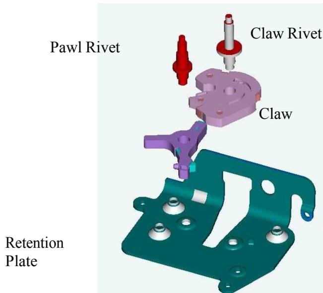
Figure 5.2, Latch assembly view. (Courtesy ArvinMeritor)
