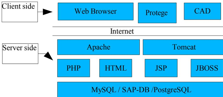
Figure 4.1, high-level view of open source server and user interface architecture
