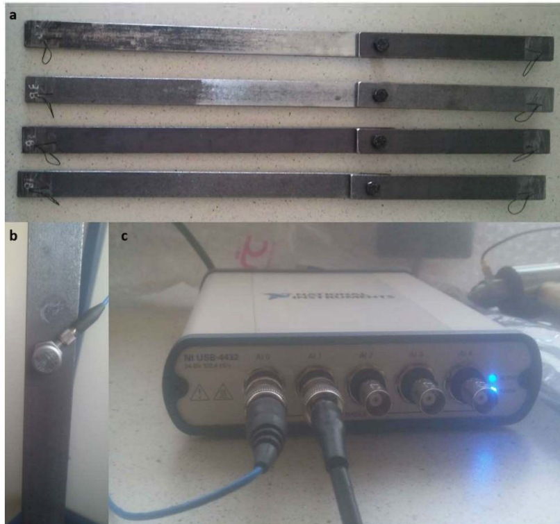
Figure 13 – Experimental test set-up: beam structures (a), accelerometer (b) and data acquisition and hammer (c)
