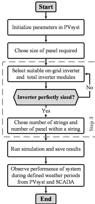
Fig. 2. The flow diagram used for performance evaluation.
