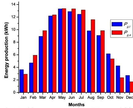
Fig. 4. Monthly energy output from PVsyst and SCADA.
