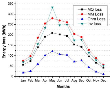
Fig. 7. Detailed System losses of the designated system
