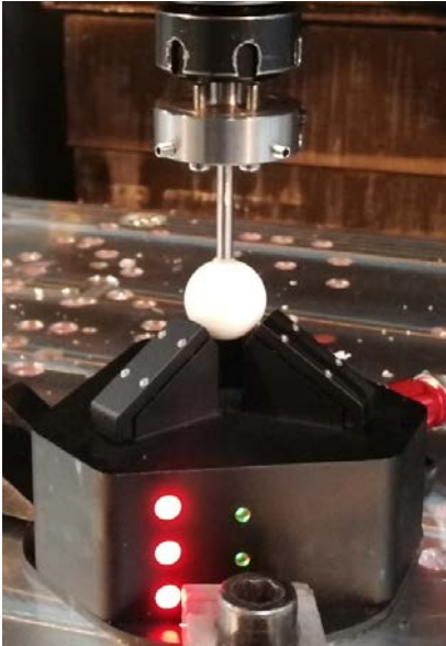
Fig.12 The prototype of non-contact R-test.
