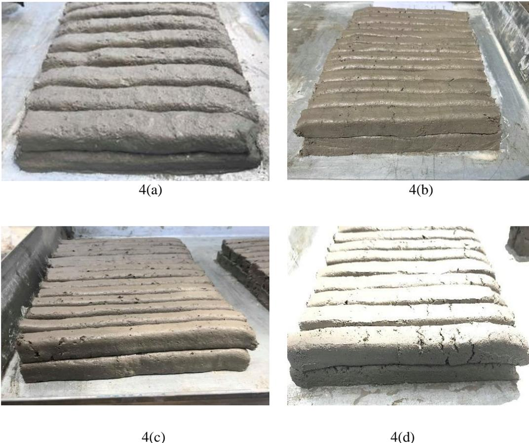
Figure 4: (a) Extruded specimen of PP 0.5%, (b) Extruded specimen of PP 1.0%, (c) Extruded specimen of PP 1.5%. (d) Extruded specimen of PP 2.0%
