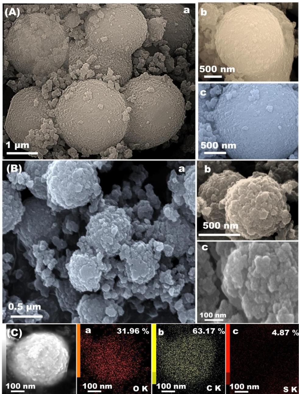
**Figure 1.** A) FE-SEM-images of the S-CSN-2 with low magnification (a). b&c) High focusing FE-SEM-images on outer surface topography of S-CSN-2. B) The FE-SEM-image of S-CSN-1 at low magnification (a). b&c) High FE-SEM magnification, focusing on the surface texture and obtaining stocked layer-by-layer formation of 3D-circular surface curvature of S-CNS-1. C) EDX-SEM mapping of S-CSN-2 of C (a), C (b), and S (c).
