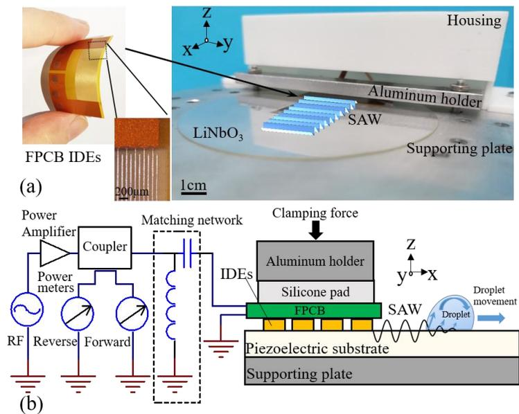
Fig. 1. (a) A photo of the FPCB IDEs and the FPCB-SAW device consisting of a FPCB stacked on a LiNbO<sub>3</sub> substrate. (b) The assembly diagram of the SAW generation on the FPCB-SAW device and its driving circuitry.
