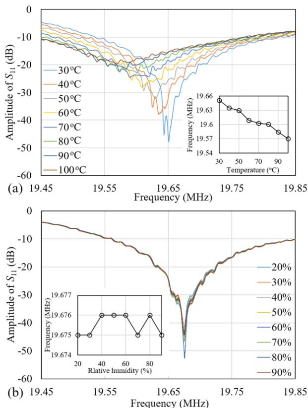
Fig. 3. Temperature and humidity tests of the FPCB-SAW device. (a) The amplitude of  $S_{11}$  changes with respect to the frequency over a temperature range of 30-100 °C. The inset is the varying Rayleigh mode frequency versus the temperature. (b) The amplitude of  $S_{11}$  changes with respect to the frequency
