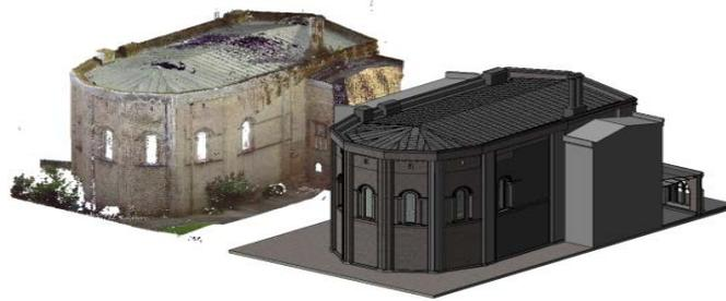
Figure 3: Point cloud data of Chapter House, Durham Cathedral and resulting BIM.
