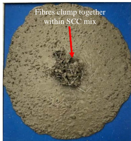
Fig. 5: Balling effect of fibres in the SCC mixtures.
