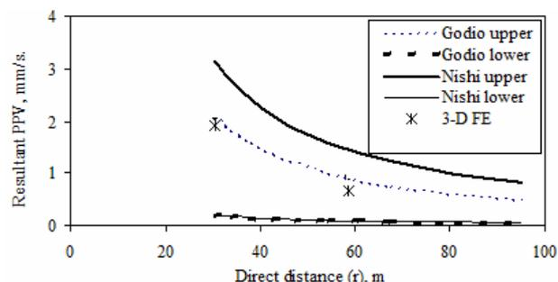
Fig. 14 3D-FE, empirical and measured PPV values at Section 3
