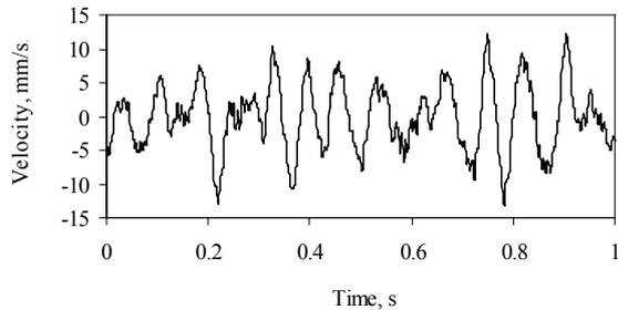
Fig. 6 Measured TBM excitation at measuring Section 1; transverse direction
