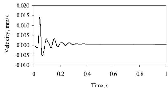
Fig. 4 Predicted time history in surface level at measuring Section 1; transverse direction
