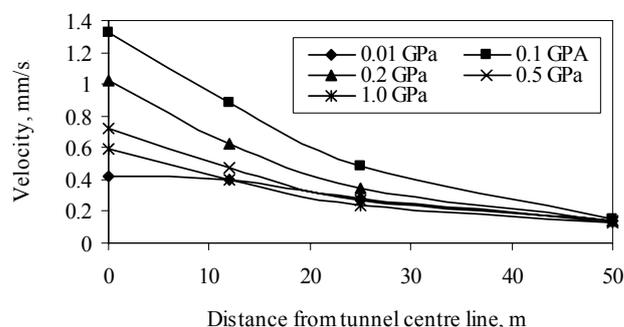
Fig. 18–The effects of stiffness on ground surface vibration
