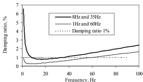
Fig. 19 Damping ratio of 0.01 (1%) dependent on frequency
