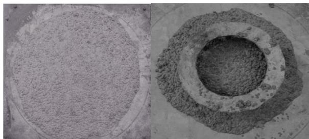
**Figure 2.** Typical slump flow and J-ring appearance.
