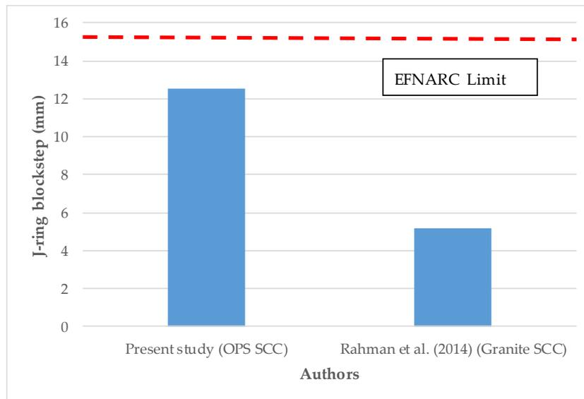
**Figure 5.** J-ring block step comparison.
