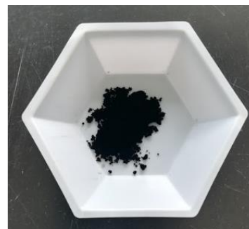
Figure 2. b) Physical appearance of multiple-walled carbon nano tubes (MWCNTs)
