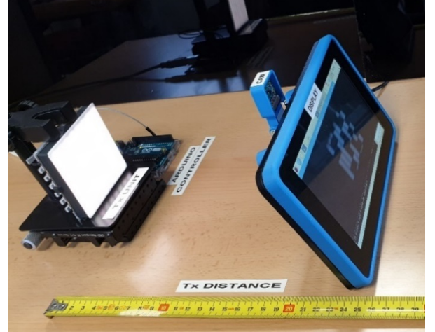
Fig. 5. Experiment setup of MIMO-OCC scheme.
