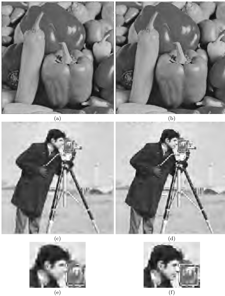
Fig. 4 Subjective evaluation of EZW-SC and EZW algorithms for Peppers and Cameraman images: (a) The Peppers image reconstructed by the original EZW with PSNR of 28.39 dB at 0.25 bpp. (b) The Peppers image reconstructed by EZW-SC with PSNR of 29.95 dB at 0.25 bpp. (c) The Cameraman image reconstructed by the original EZW with PSNR of 23.41 dB at 0.25 bpp. (d) The Cameraman image reconstructed by EZW-SC with PSNR of 24.52 dB at 0.25 bpp. (e) An enlarged part of the Cameraman image reconstructed by EZW. (f) An enlarged part of the Cameraman image reconstructed by EZW-SC
