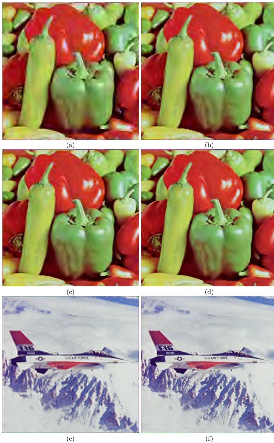
Fig. 7 Subjective assessment of three codecs: the proposed CEZW-SC, the method reported in [35] and CCEZW [11] for Peppers and Airplane colour images: (a) The Peppers image reconstructed by the original CCEZW with PSNR of 22.79 dB at 0.125 bpp. (b) The Peppers image reconstructed by CEZW-SC with PSNR of 24.67 dB at 0.125 bpp. (c) The Peppers image reconstructed by the the original CEZW with PSNR of 25.15 dB at 0.25 bpp. (d) The Peppers image reconstructed by CEZW-SC with PSNR of 27.15 dB at 0.25 bpp. (e) The Airplane image reconstructed by the method reported in [35] with PSNR of 26.6 dB. (f) The Airplane image reconstructed by CEZW-SC with PSNR of 30.99 dB
