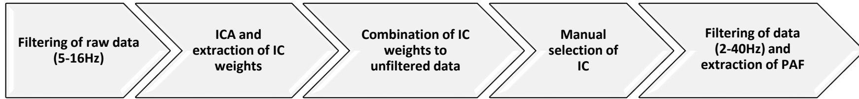
Figure 2: Diagram of the PAF extraction. After filtering raw data, an independent component analysis (ICA) was performed, followed by the extraction of the corresponding IC weights.
